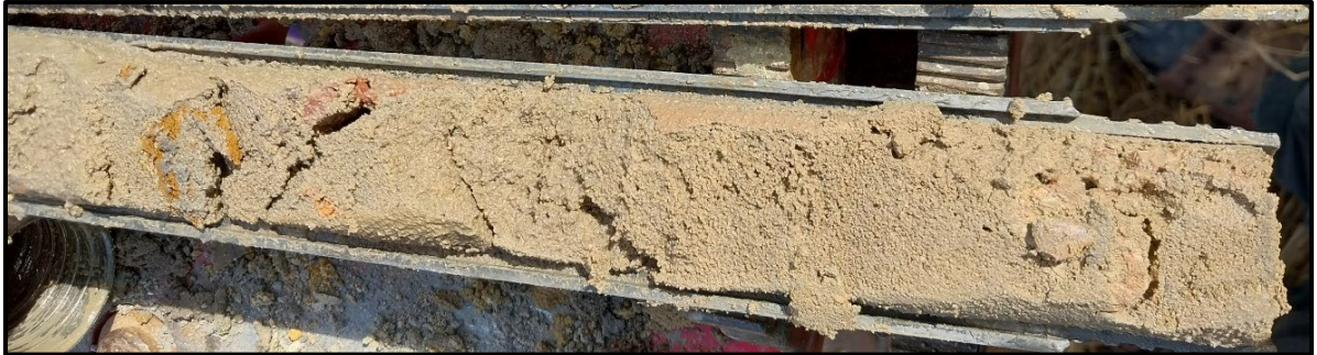
Figure 4-3. Young Alluvial Flood-Plain Deposits in Boring B-2
